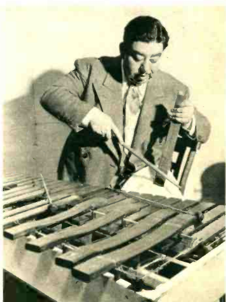
The marimba poses a real problem, must usually be sent back to the factory. Expert Jose Bethancourt shows how wooden keys are filed.
